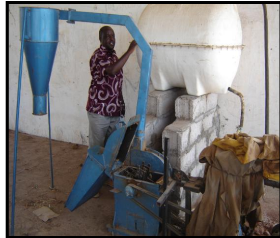
Pods can be milled into flour using small village mills
